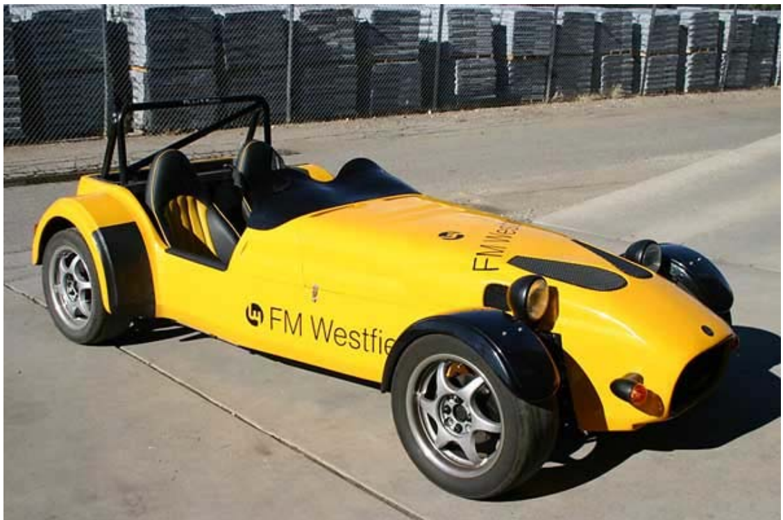
"Aeroscreen" aerodynamic windscreen.
