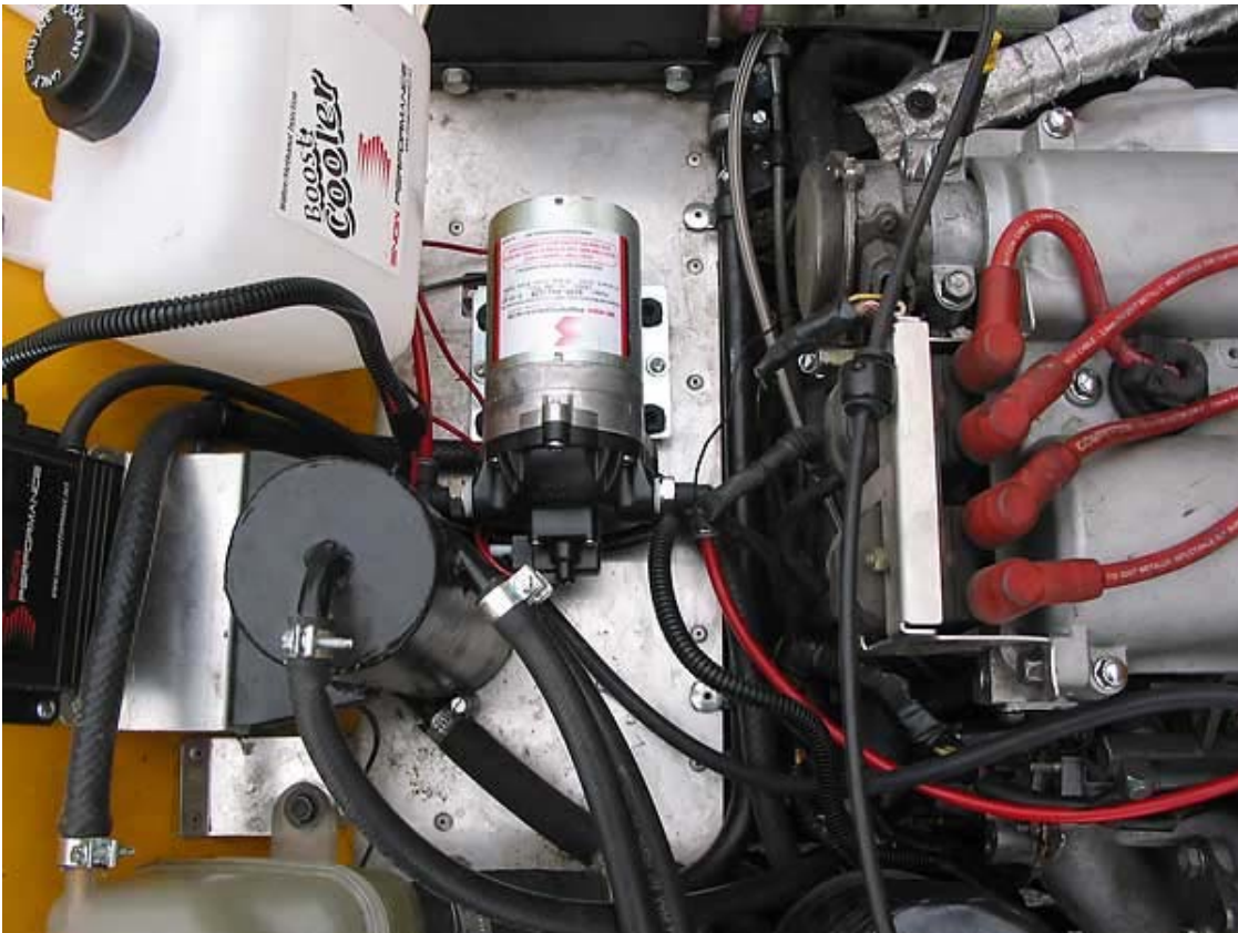
Black canister (left) is a swirl pot / reservoir for the fuel system.
