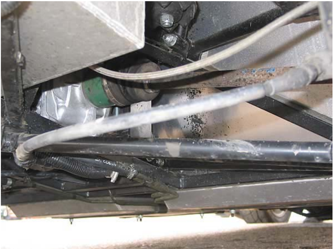
Independent rear suspension... using Mazda Miata halfshafts and CV joints.
