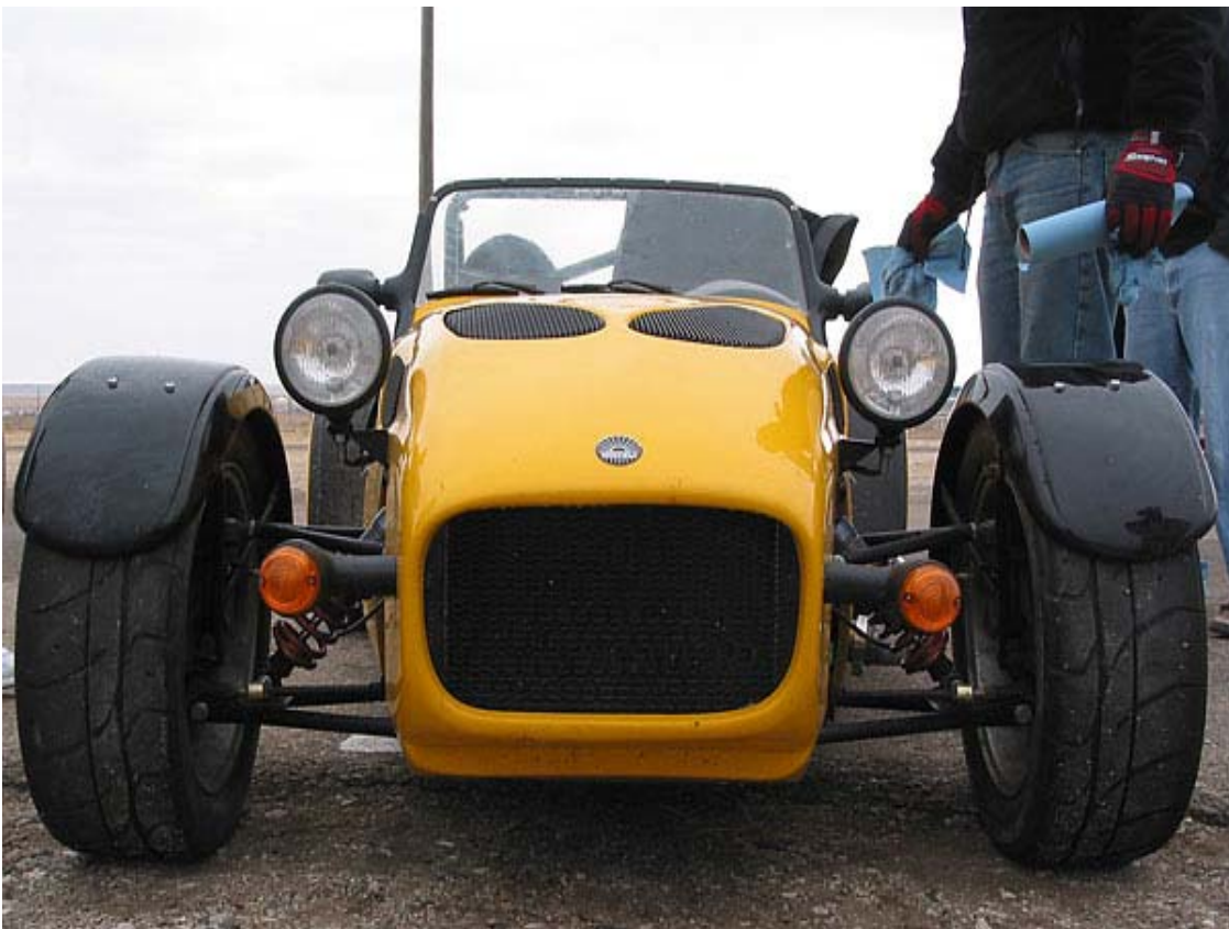
This car has the optional one-piece nose. Two-piece (nose plus bonnet) is standard equipment.
