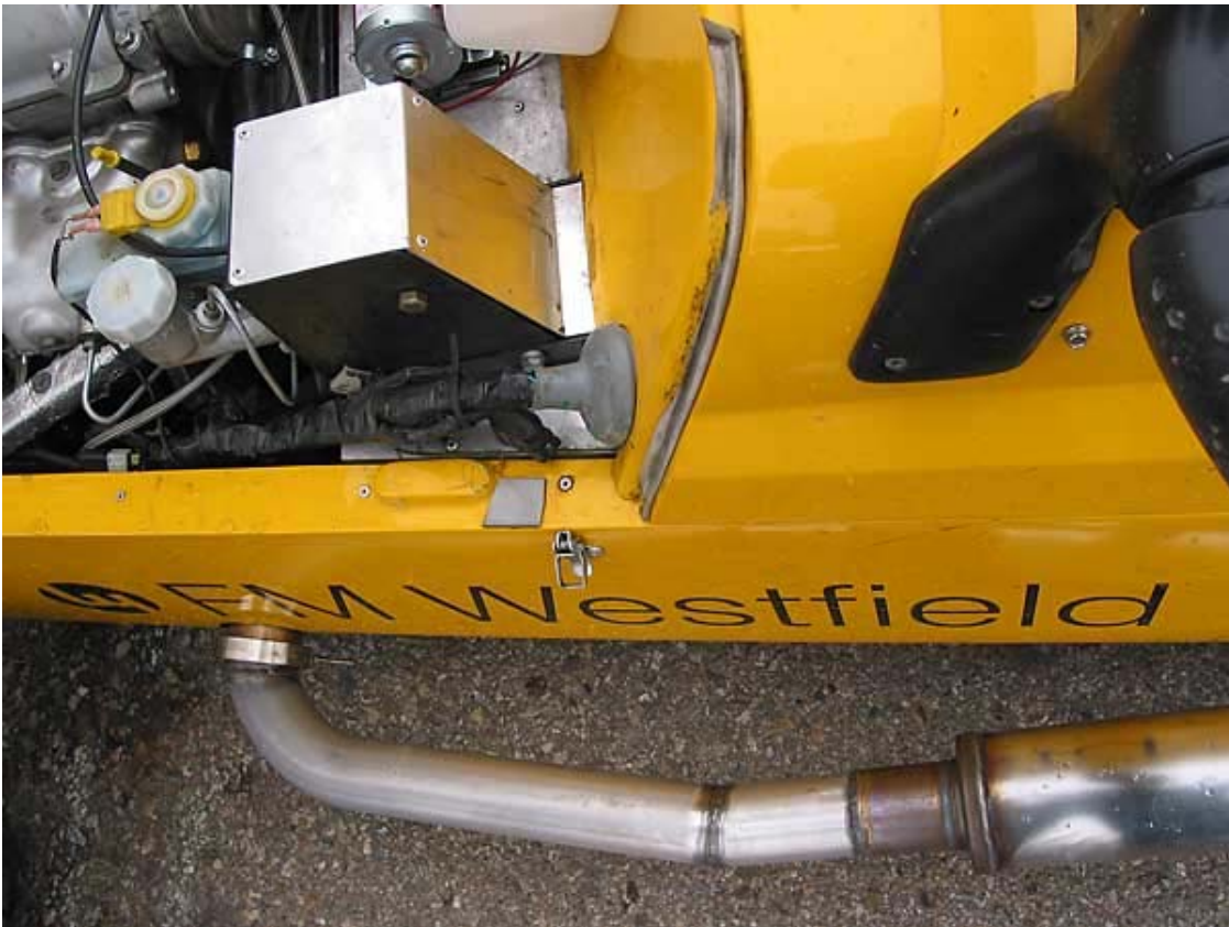
Custom fabricated exhaust downpipe... notice the V-band attachment.
