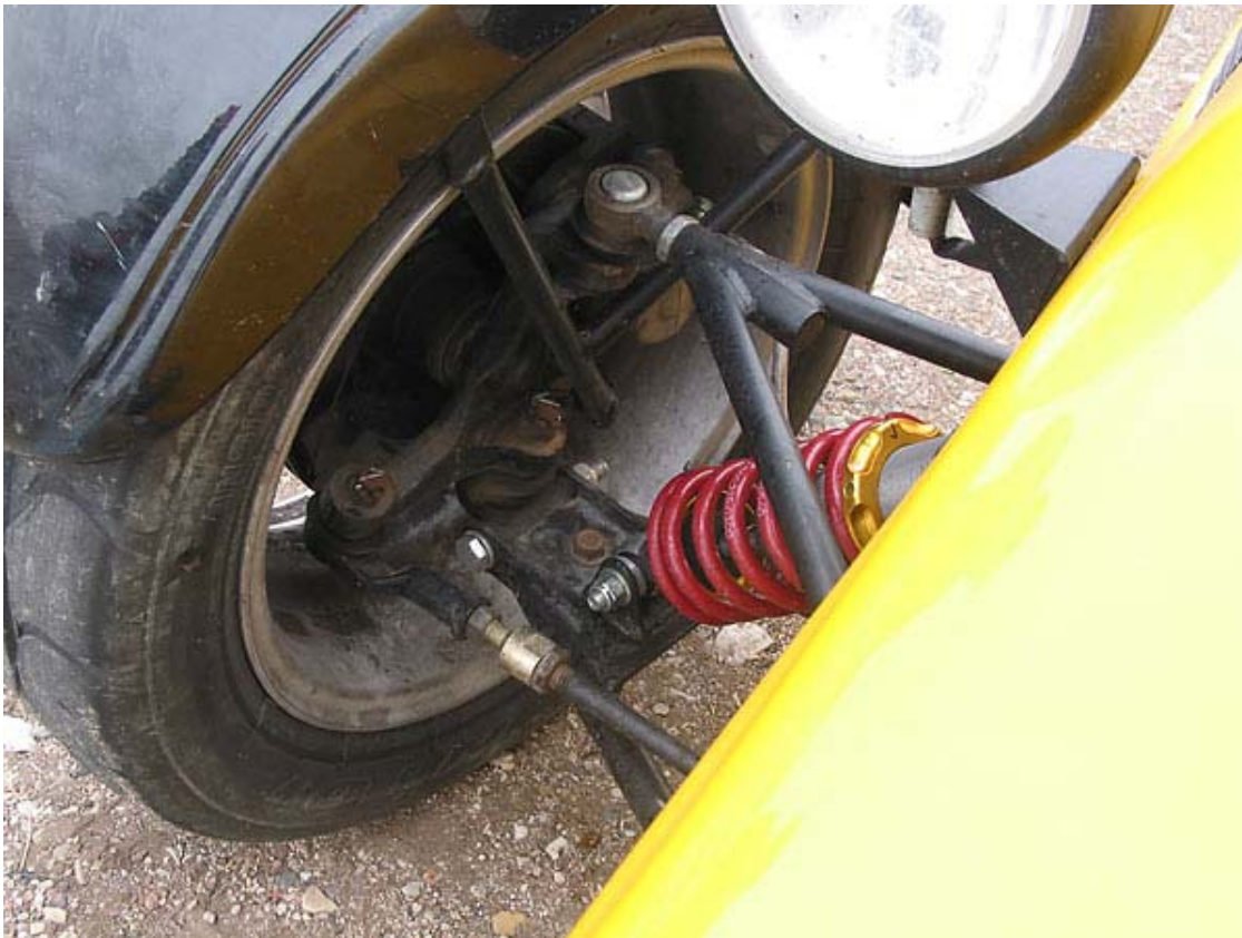
The Westfield kit is designed to use Miata donor parts, like uprights and brakes.
