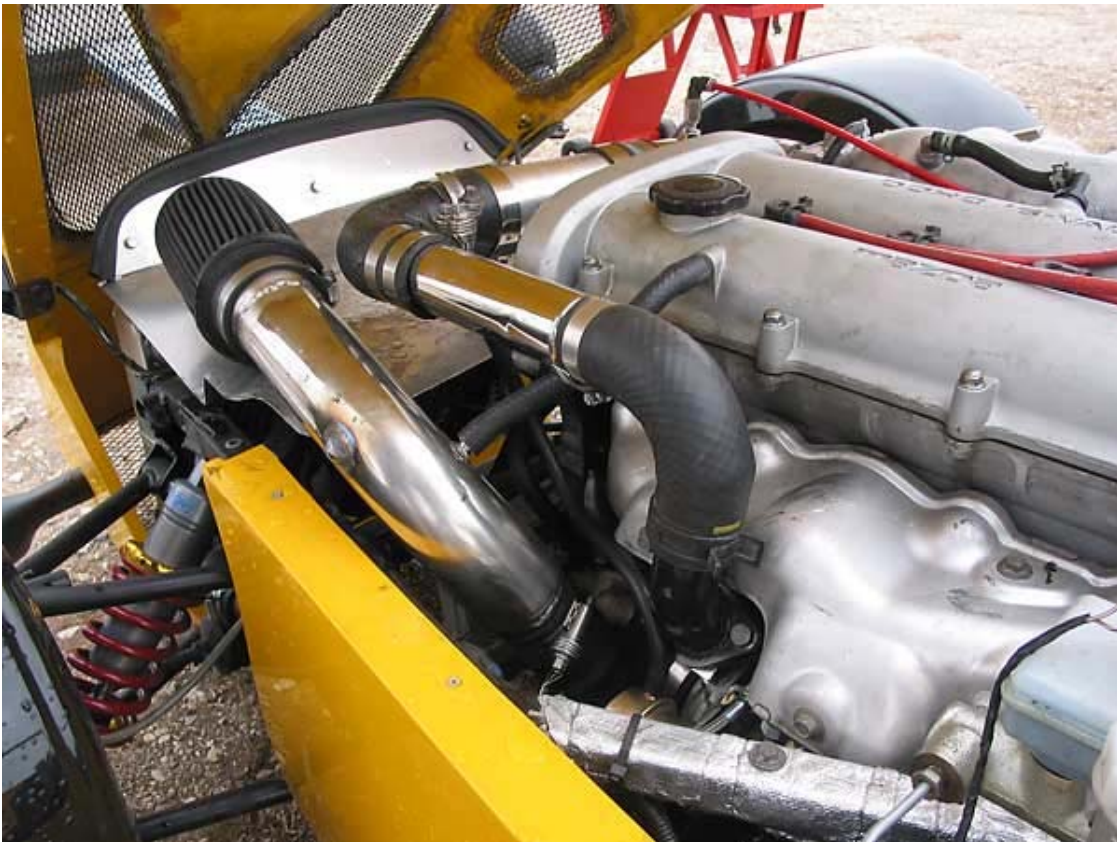
Red tube (top) is for the water injection system.
