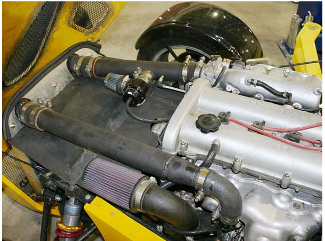
Intercooler plumbing. Note also that the air filter gets cool air through a hood vent.
