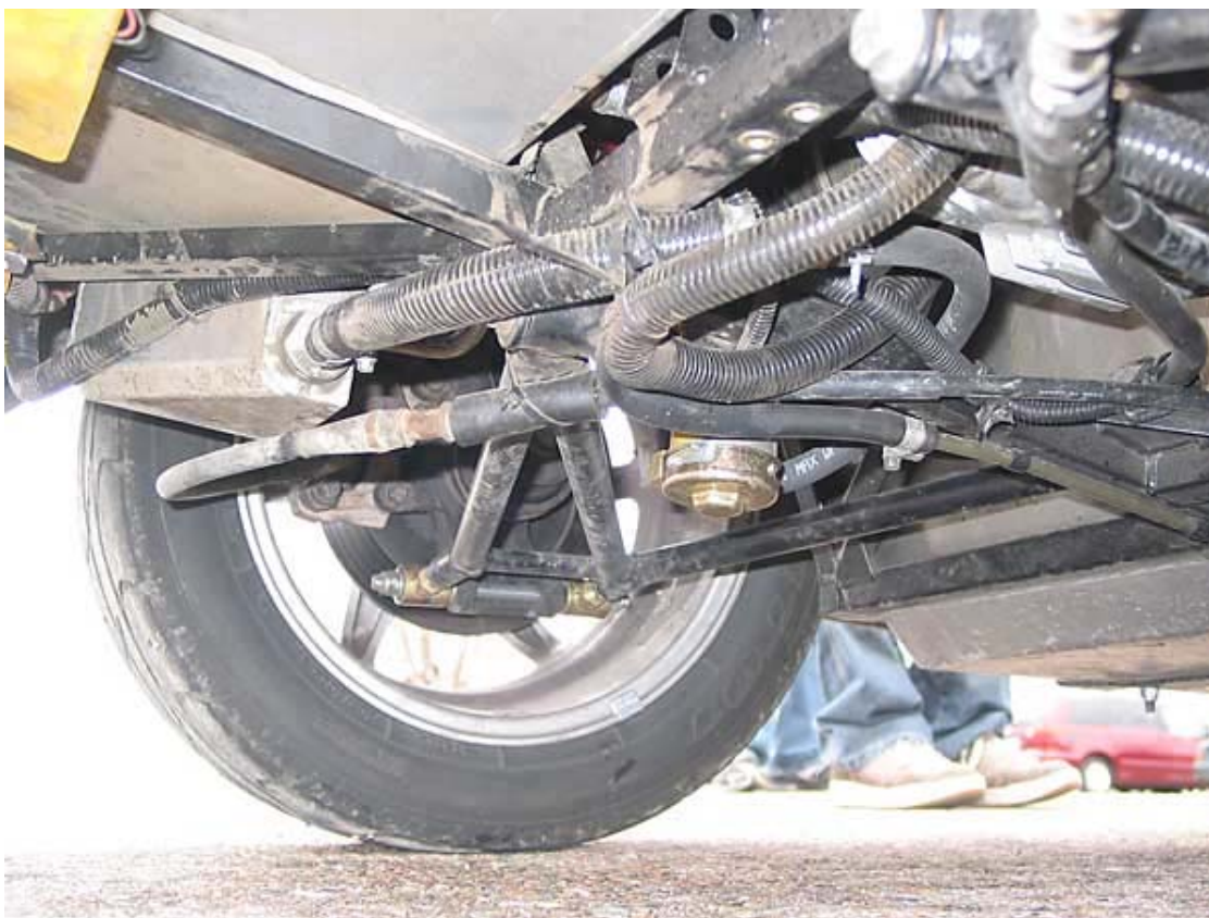
Facet fuel pump shown here is the low pressure supply to the scuttle-mounted swirl tank. (The high pressure pump for the fuel rail is mounted next to one of the motor mounts.) Standard fuel tank (here) is 7.5 gallons. A larger 11.9 gallon tank is available.
