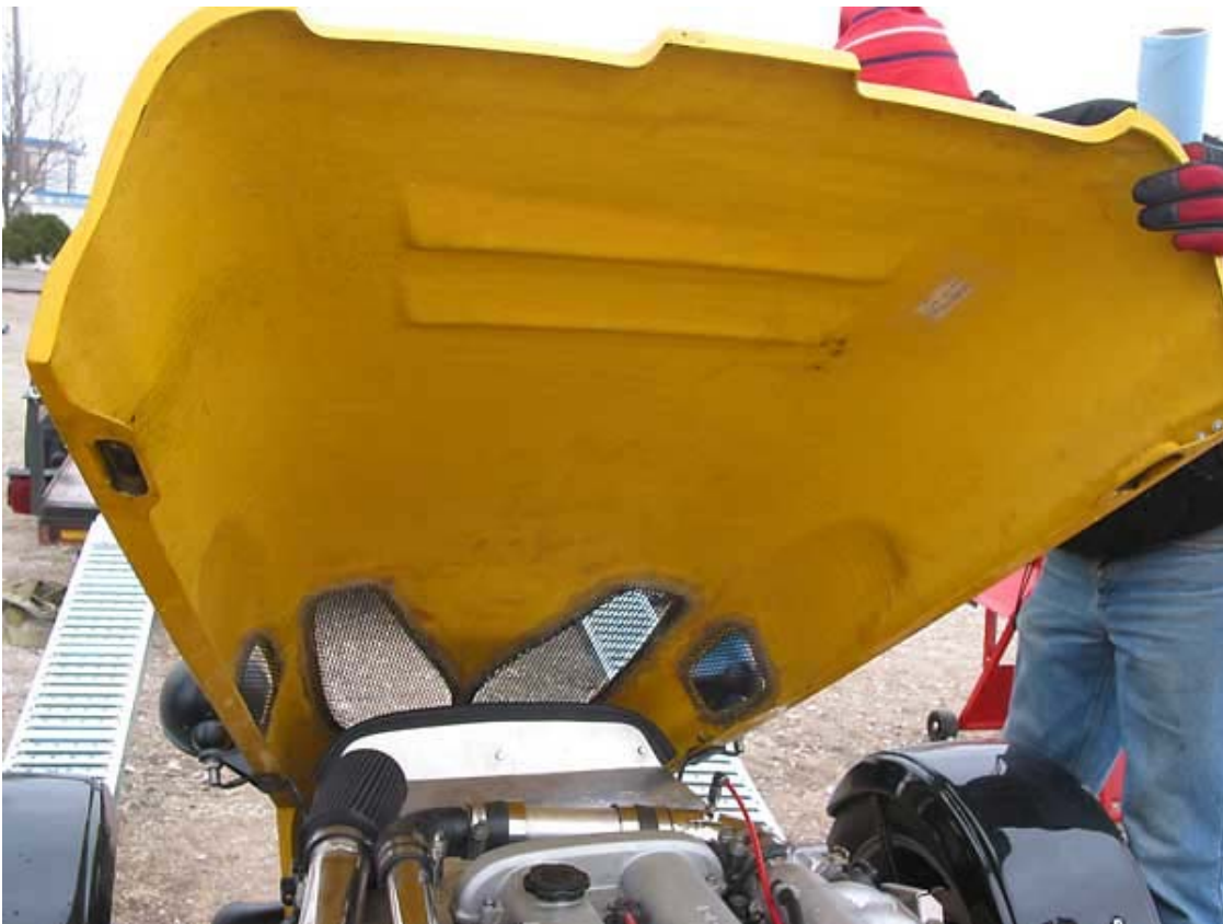
The fiberglass body panels are molded in color, so their beauty is more than skin deep! (Paint is optional.)
