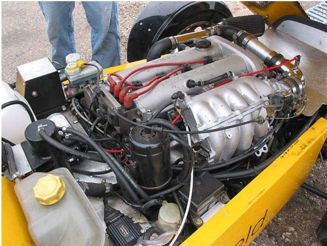
A compact Odyssey PC680 battery has been relocated from the scuttle (here) to the passenger-side foot box.
