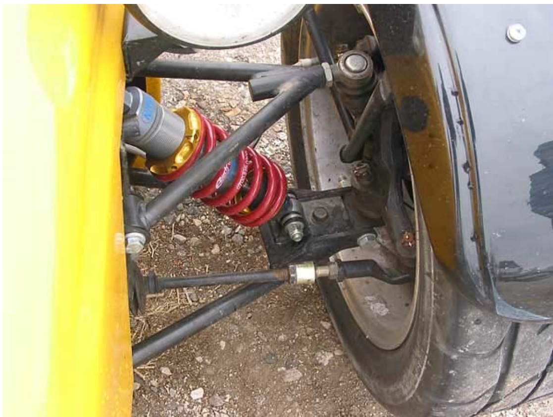
Westfield provides threaded adapters so that their rack will work with Miata tie rod ends.
