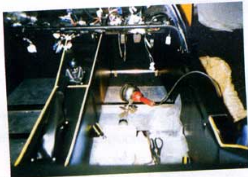
Removal of interior after MOT to introduce additional circuitry for interior lights, shift light etc.
