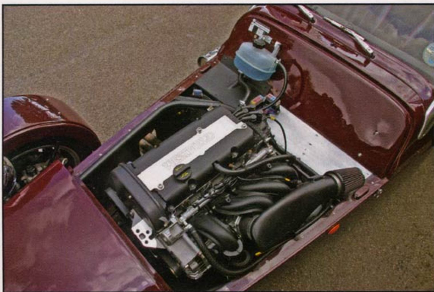
The proven Ford Zetec engine--1600 (left) and 1800 (right) is readily available both in Europe and America. Ford racing even sells crate engines and hop-up parts for these mills.
