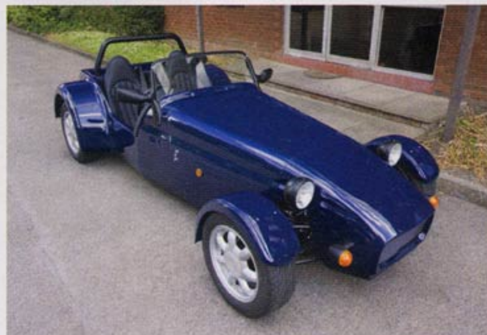
The new SDV-M is based on Mazda MX-5 running gear. Note Miata wheels. This should be a very popular kit.
