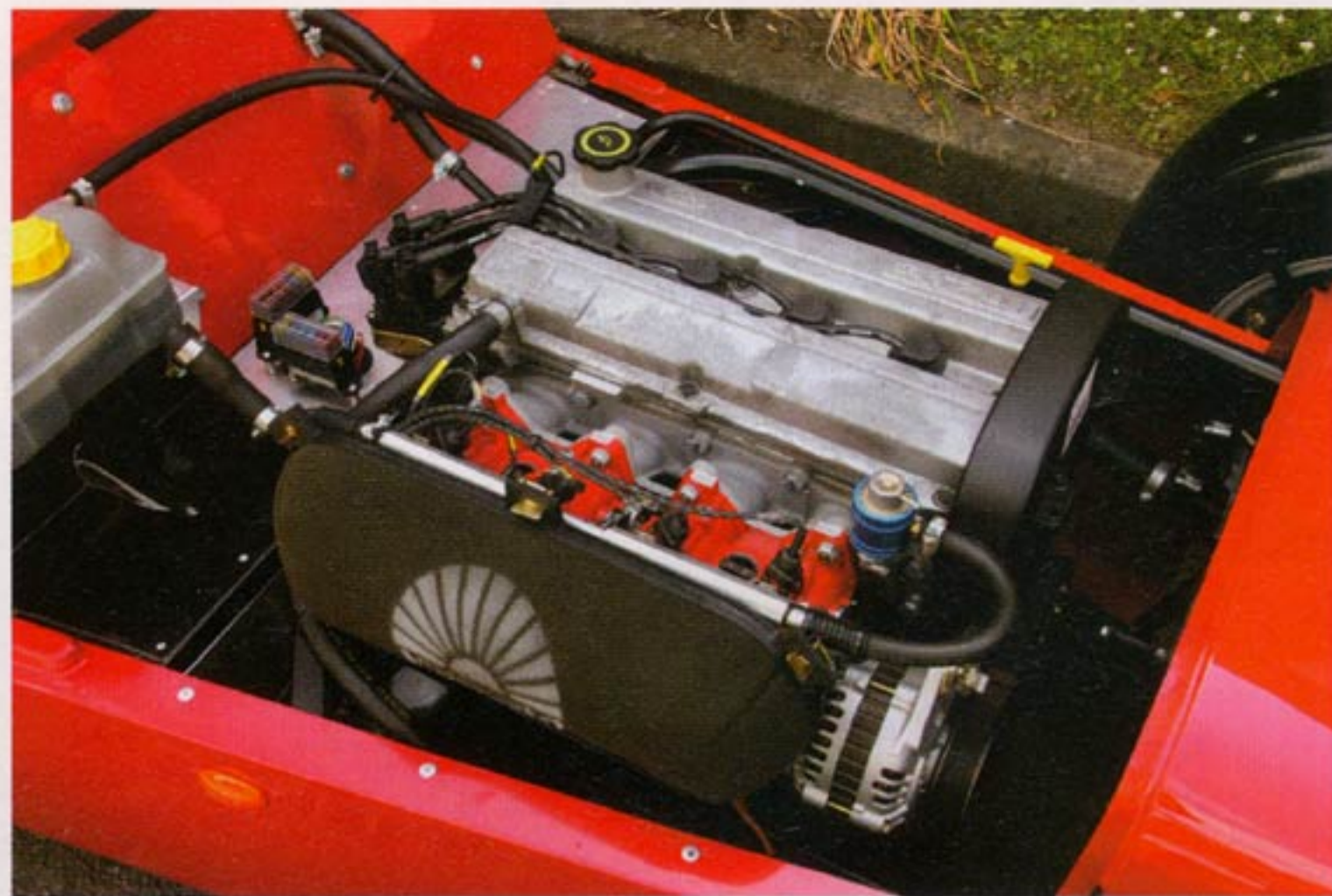
The proven Ford Zetec engine--1600 (left) and 1800 (right) is readily available both in Europe and America. Ford racing even sells crate engines and hop-up parts for these mills.
