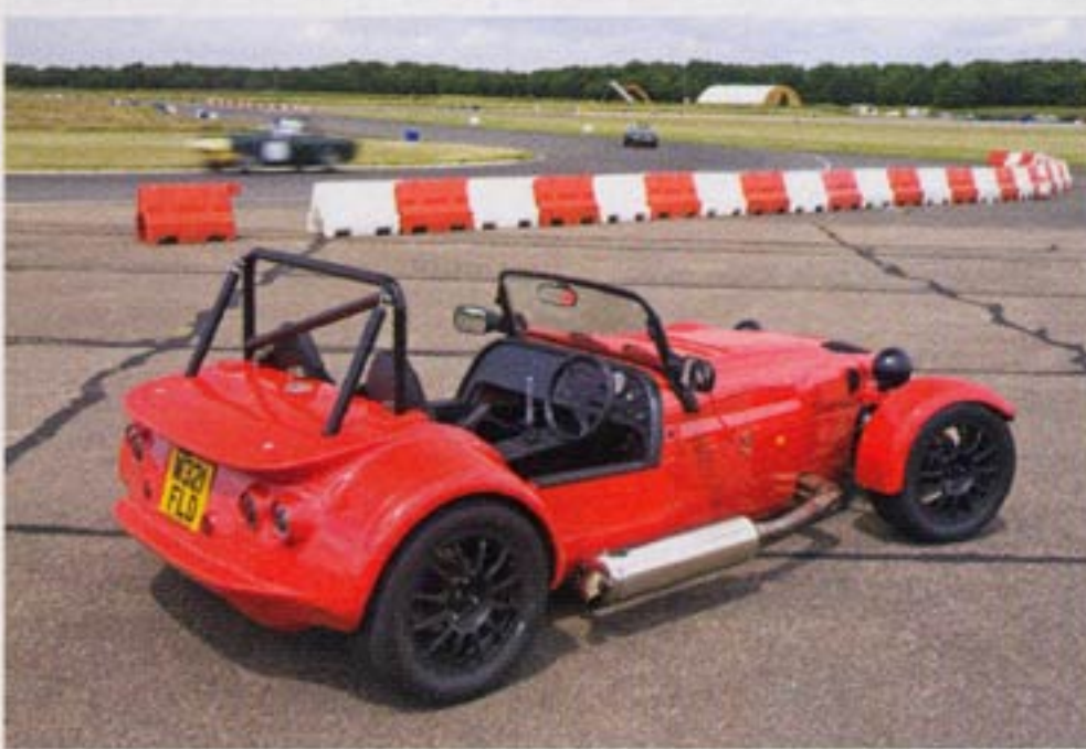
The Sport 2000S FW body (top and above) has this sporty tail with molded-in quad tail lights, spoiler and diffuser slot.
