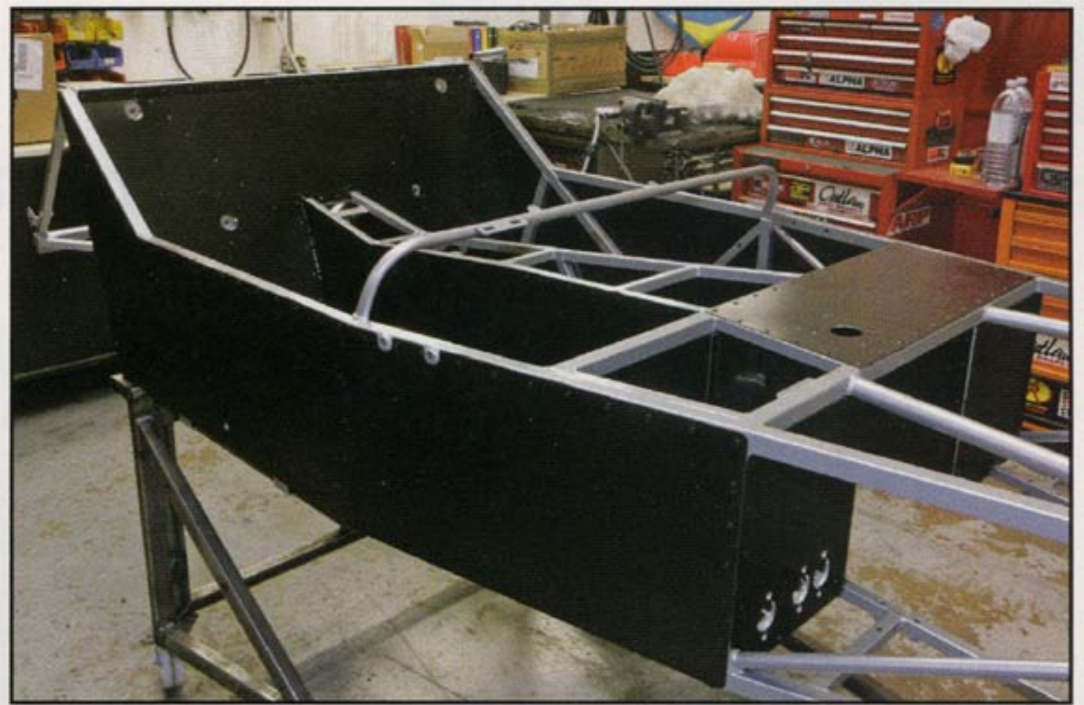
Turnkey cars are paneled up in aluminum. The rivet holes are laser-cut so replacement panels can be attached directly to existing holes.
